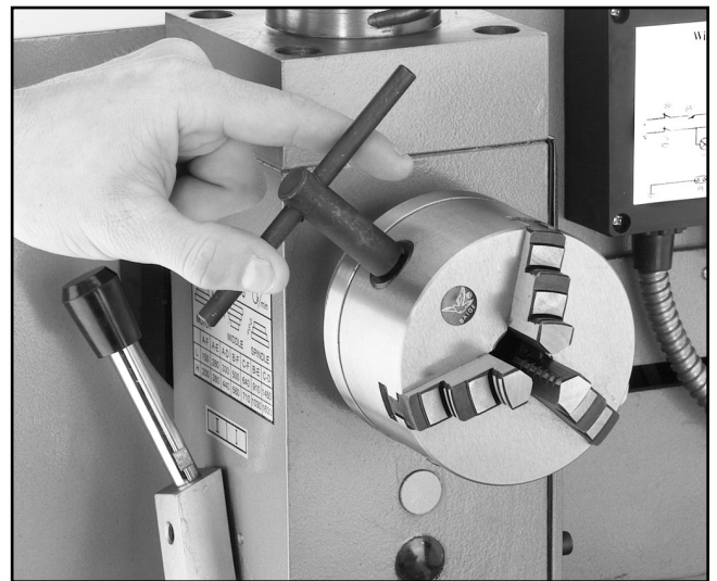
Figure 6. Rotate chuck key to open/close jaws.
